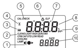
1. The measuring scheme (lamp, cuvette, detector), appears during different phases of zero or reading measurement
