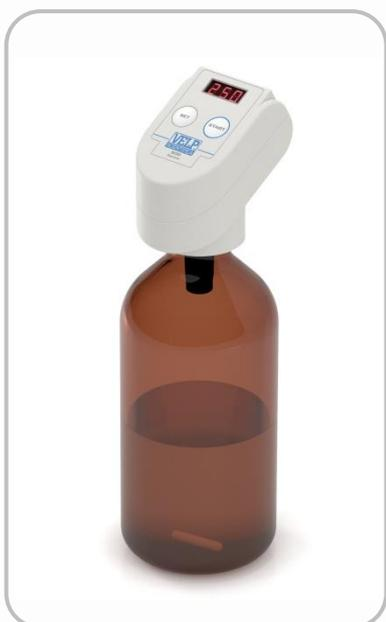
The BOD Sensor Set is a **ready-to-use solution** consisting of a BOD Sensor, a dark glass bottle, an alkali holder to absorb the carbon dioxide and a stirring bar.
